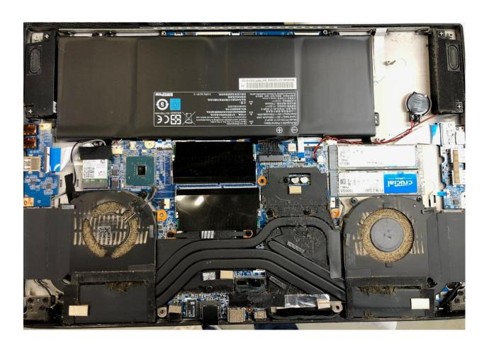
Remove the 3 screws and the plug holding in the fan. Also, cut one or both sections of tape holding down the fan to either pull back the fan or pull out the fan. We will also be removing the fan cable, you will need to pull out the plug by pulling it out towards the fan (see below images)
