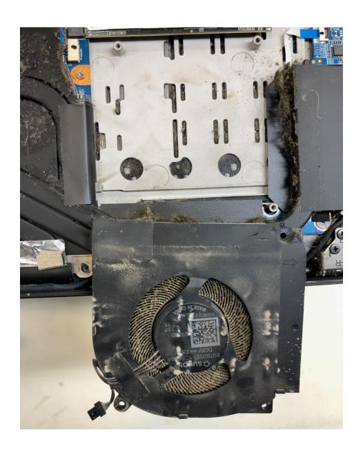
Clean out the fans, you can pick out the dust and then spray out the fans the rest of the way with compressed air or use a toothbrush.
