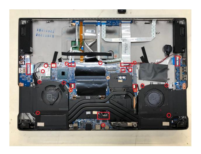
After the screws are removed the motherboard can be lifted off. ADVISE, there is a power cable going from the motherboard to the button.
