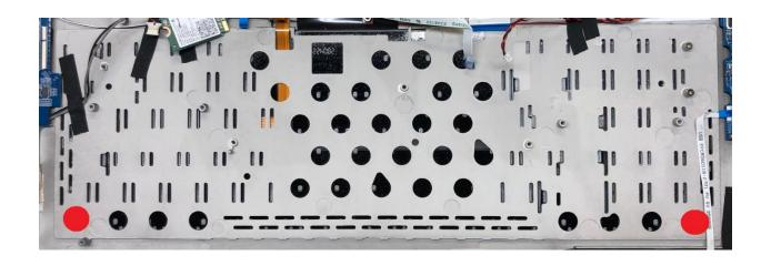
Prior to installing the replacement keyboard all prior keyboard debris should be removed and you should be left with a 'white' backing that it will be adhered to.
