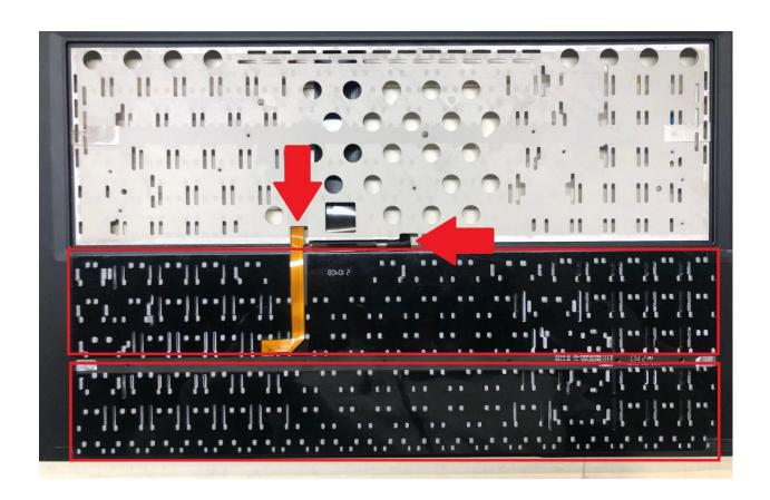
After removal of the keyboard liner lift it up at a 90 degree angle and slide it left and right.
