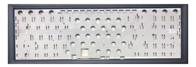
Upon reinstallation of the keyboard, we would recommend not taking off the liner until keyboard cables are routed properly into the chassis prior to taking off the lining.
