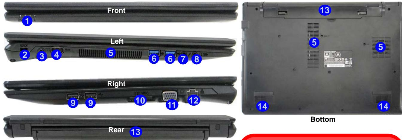
Figure 7 - Front, Left, Right, Rear & Bottom Views (Model B)
