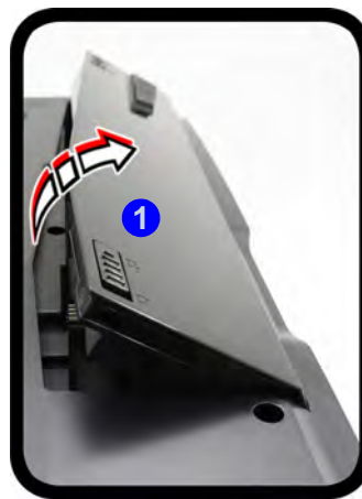
Figure 27 - Remove the battery and Insert the USIM Card
