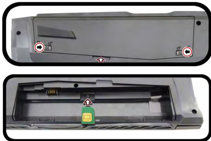
Figure 27 - Remove the battery and Insert the USIM Card
