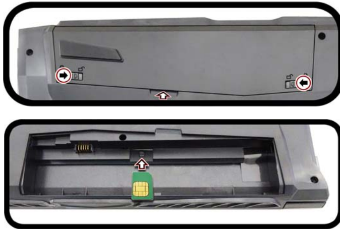
Figure 29 - Remove the battery and Insert the USIM Card
