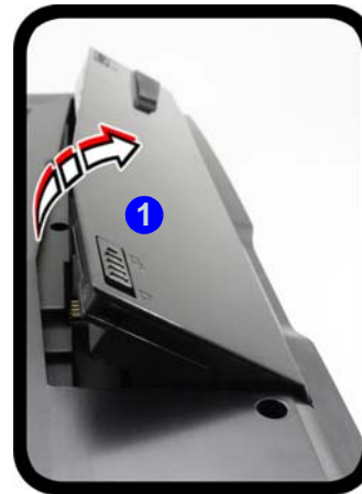
Figure 31 - Remove the battery and Insert the USIM Card
