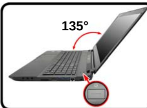
Figure 1 - Opening the Lid/LCD/Computer with AC/DC Adapter Plugged-In
